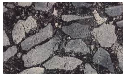
Abrasive grains of same size but with heavier bond coating and thicker, stronger bond posts as in a hard grade wheel.
