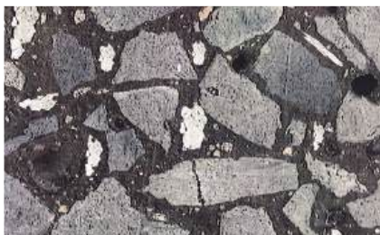
Abrasive grains with light bond coating and weak connecting bond posts as in a relatively soft grade wheel. (Bright areas are the pores, required for chip clearance).
